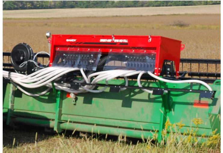
For mounting, the 1018 No-Till Orbit-Air comes with a sturdy 2-1/2" x 2-1/2" square steel mounting frame. Allows unit to be bolted or secured with U-bolts to a customer supplied mounting platform.
