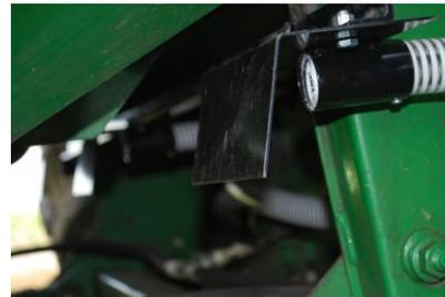
An 18-outlet deflector package includes deflectors and angle iron mounting straps to
